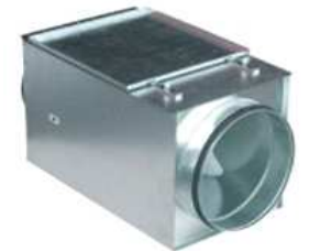
5416744600 - MFL-100 F Box in galvanized steel for inserting the MFR F5, F6 and F7 filters. Fitted with inlet and discharge circular duct connection flanges with integrated rubber air seal and an inspection cover easy to open for maintaining the filters.
